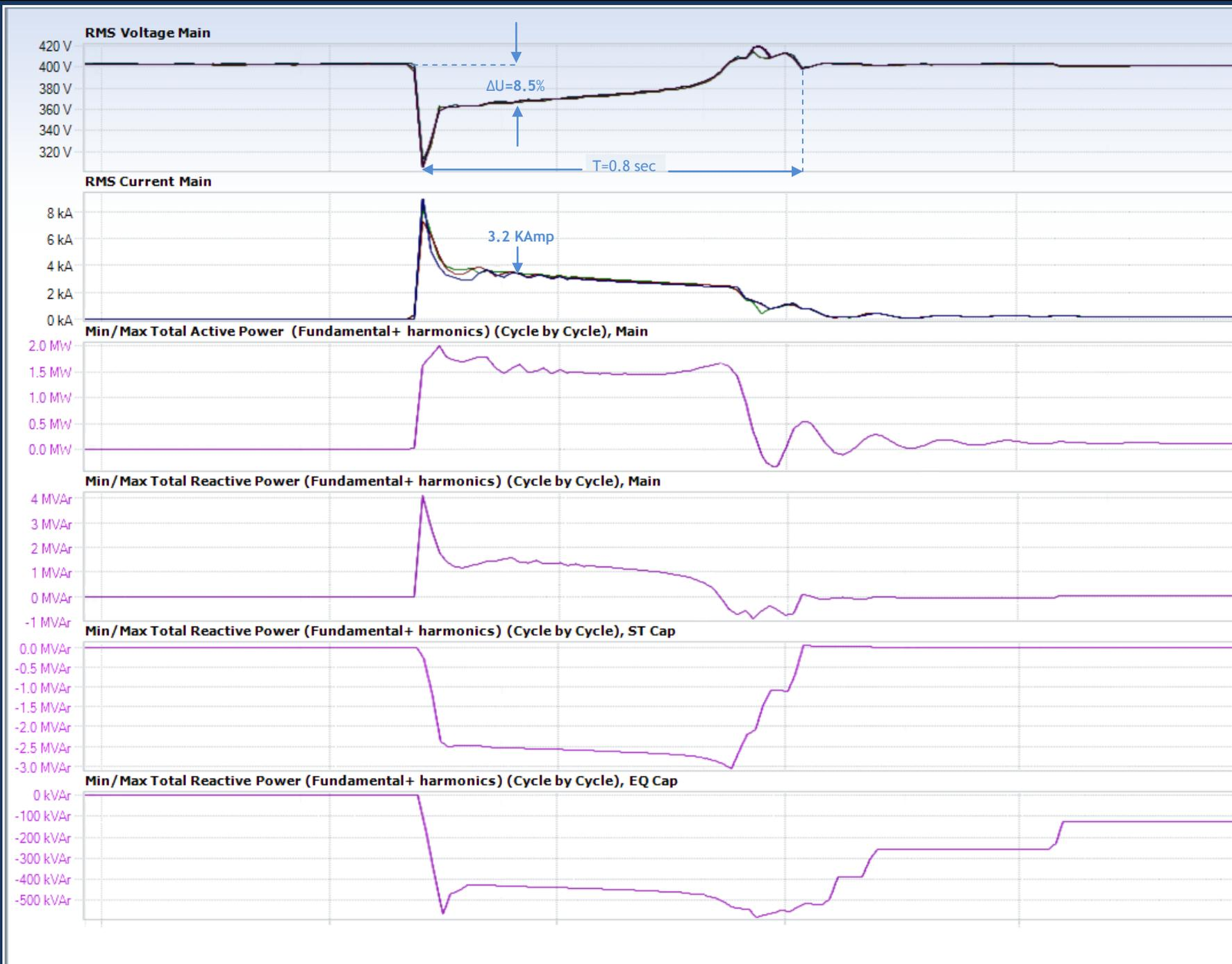
Figure 3b: Motor Startup With EQ-ST & EQ Compensation
